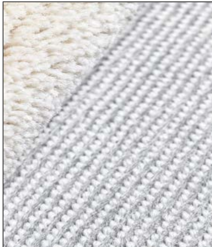
Fig. 10: non-woven primary backing from below, no backing
