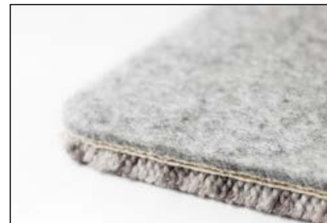
Fig. 12: non-woven secondary backing from below
